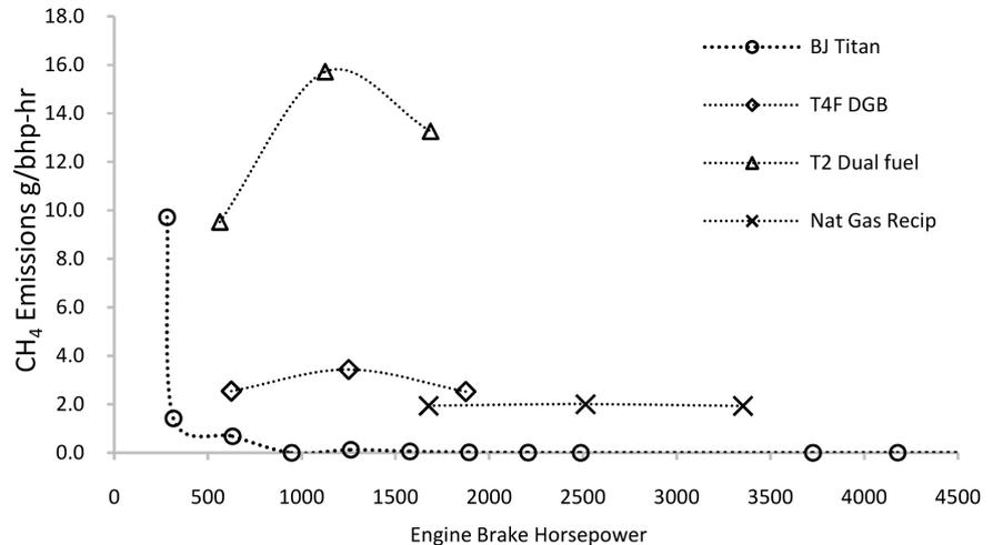
**Figure 4.** Methane slip from emissions test on TITAN turbine at increasing load compared to OEM reported methane slip data.
