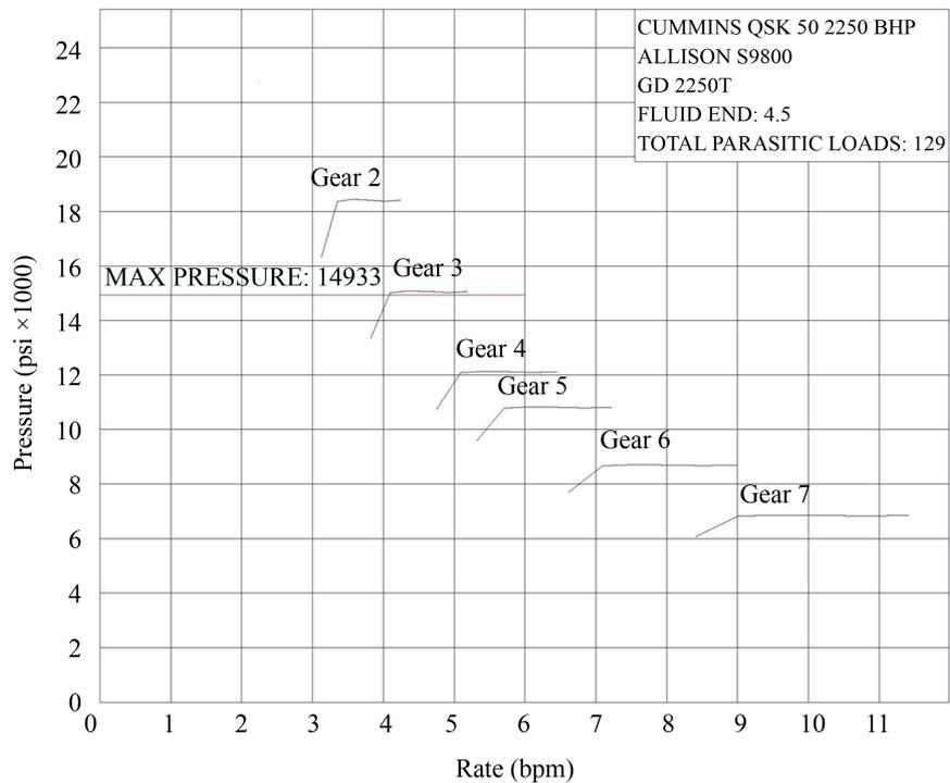
**Figure 5.** Conventional fracturing pump curve at 100% engine load varying engine RPM.
