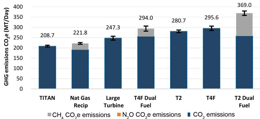
**Figure 11.** Case 1 CO<sub>2</sub>e emissions for different frac fleet technologies in Haynesville basin.
