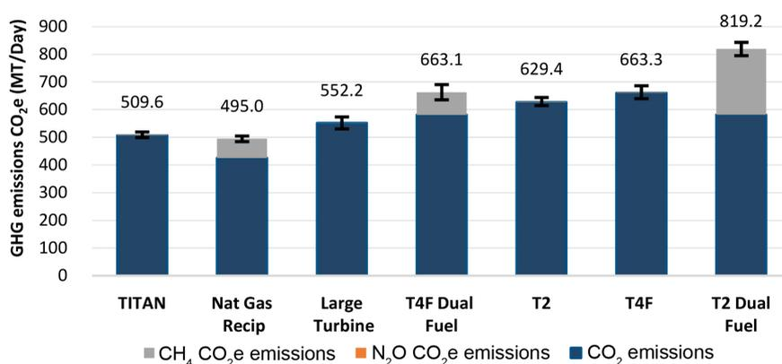
**Figure 14.** Case 4 CO<sub>2</sub>e emissions for different frac fleet technologies in Permian performing a Simulfrac.
