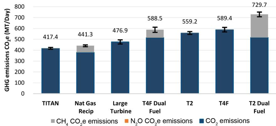
Figure 13. Case 3 CO<sub>2</sub>e emissions for different frac fleet technologies in Haynesville performing a Simulfrac.
