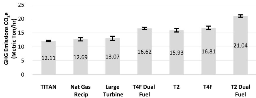
**Figure 16.** Emissions rate per pumping hour of various fracturing fleet technologies based on emissions modelling.
