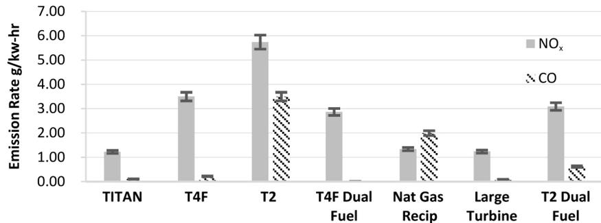
**Figure 18.** Emissions rate of NO<sub>x</sub> and CO by various frac fleet engine technologies on Case 1 engine loading.
