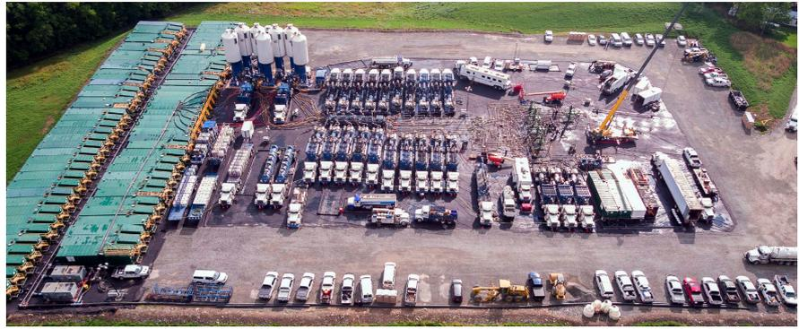
**Figure 1.** Typical hydraulic fracturing fleet with 23 diesel powered fracturing pumps and support equipment.
