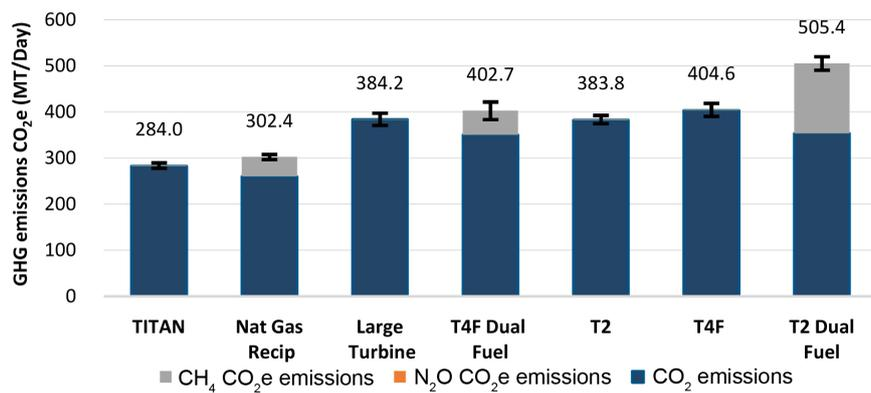
**Figure 15.** Case 5 CO<sub>2</sub>e emissions for different frac fleet technologies in Montney/Duvernay basin.
