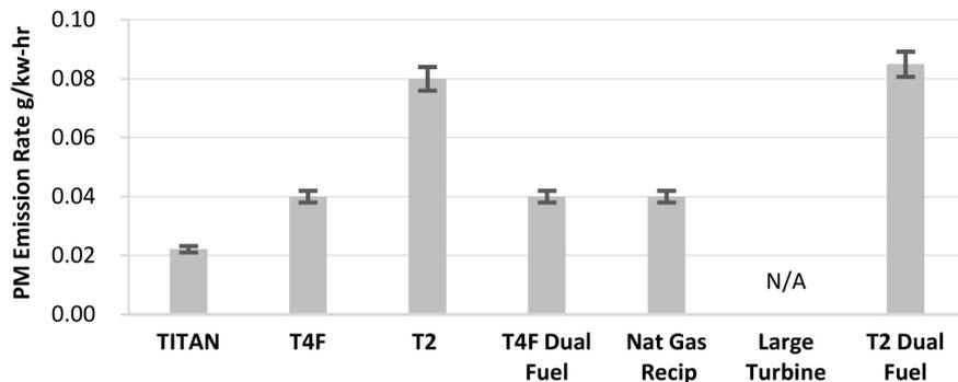
**Figure 19.** Emissions rate of Particulate Matter (PM) by various frac fleet engine technologies on Case 1 engine loading.
