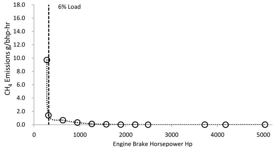
**Figure 2.** Titan CH<sub>4</sub> emissions test methane slip at various loads.
