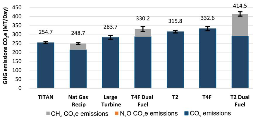
**Figure 12.** Case 2 CO<sub>2</sub>e emissions for different frac fleet technologies in Permian basin.
